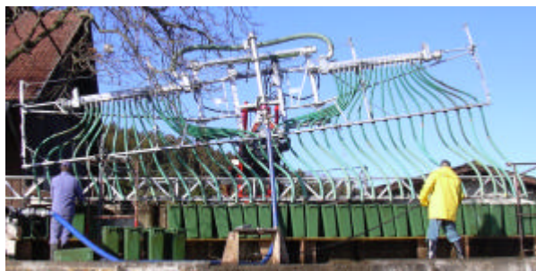
Trailing hose spreader on the test bench with 15 % gradient
